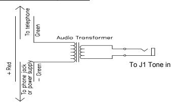
This is how you are able to insert the confirmation tones into the telephone line so that when you are dialing from a remote location you can hear the URC1 talk back to you, and let you know that a code was correctly received and processed. You may also receive tones as well with this circuit. Notice it is in parallel with the phone line instead of series like the previous circuit.
